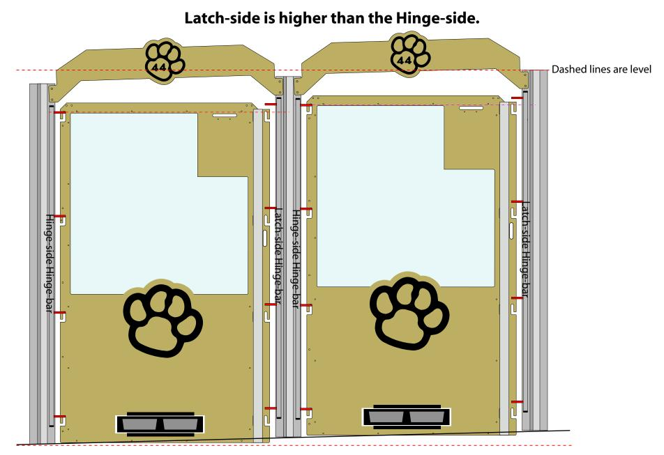
In this case the hinge-side hinge-bars need to be raised - and the latch-side hinge-bars might need to be lowered. Depending on the sevarity of the slope, the hinge-side hinge-bars need to be raised father than the post will allow (without running into the header. We have built special hinge-bars in this situation. Contact us if you run into this problem.
